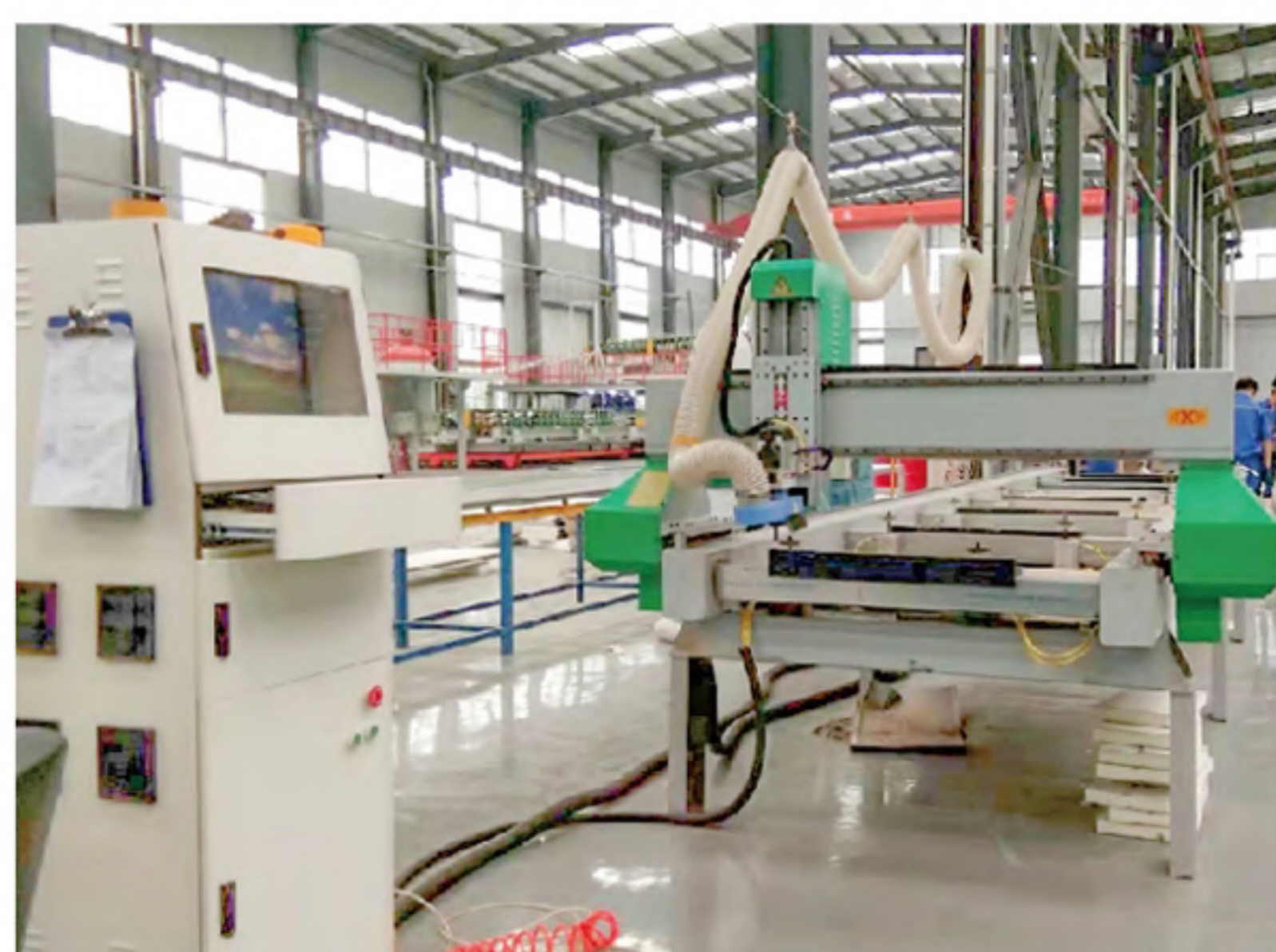
Window hole cutting and pre-drilling hole of screws
